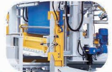
Face Mix Unit with Safe Hydraulic Locking
